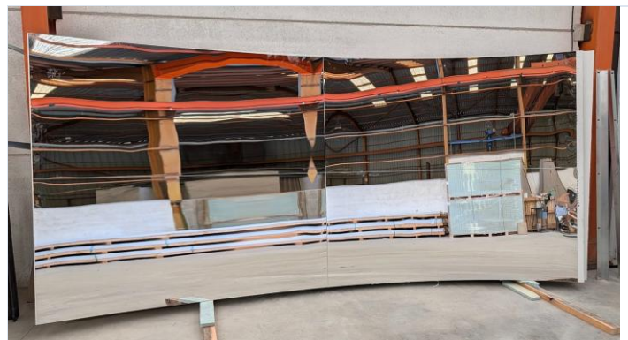
A completed composite mirror panel, the first of the series. (Credit: FERRUM)
