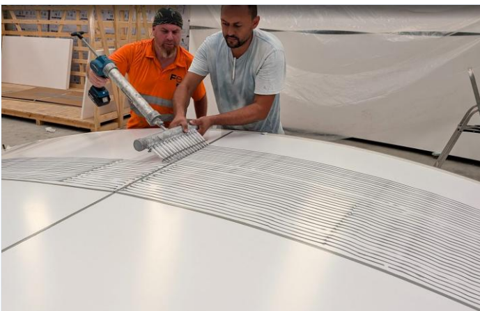
Bonding the thin-glass mirror strips onto a finished panel. (Credit: FERRUM)
