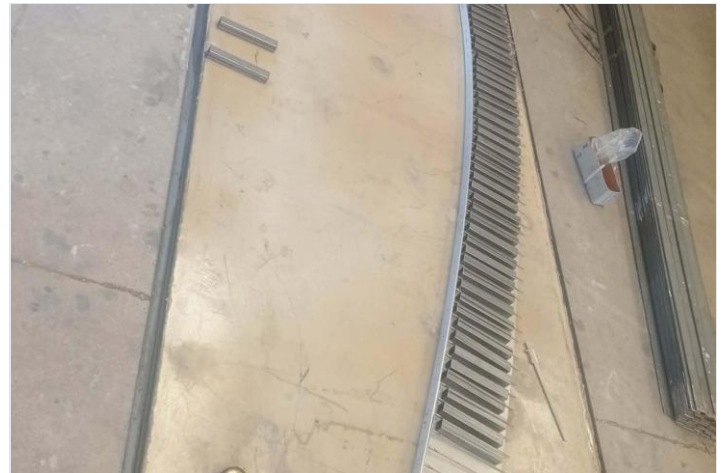
Mirror form-structure template at the production site.
