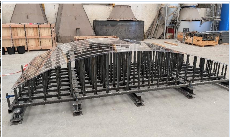
Mirror-mould prepared for sandwich-panel production.
