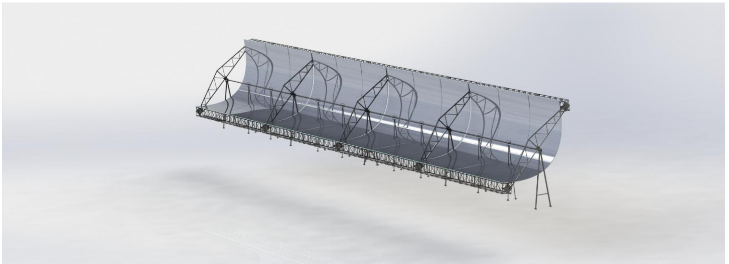
The MSA-Trough collector — a fixed-focus concentrator with a detached, continuous absorber line.
